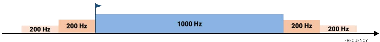
Figure 3. Marport Pro sensors (e.g. Trident, Door Explorer, all Navigator range except Catch)
