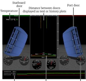
Depth of Spread diagram displays distance Pitch & roll door sensors between Port/Clump/Starboard
