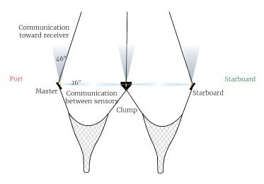
The beamwidth toward the receiver (uplink ping) is 46° and beamwidth toward the other sensors (down ping) is 26°. This beamwidth is thinner: this is why it is important to keep sensors aligned.
