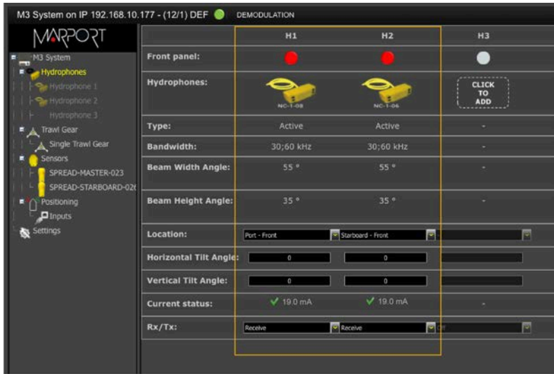
Figure 6: Hydrophone configuration for Spread sensors
